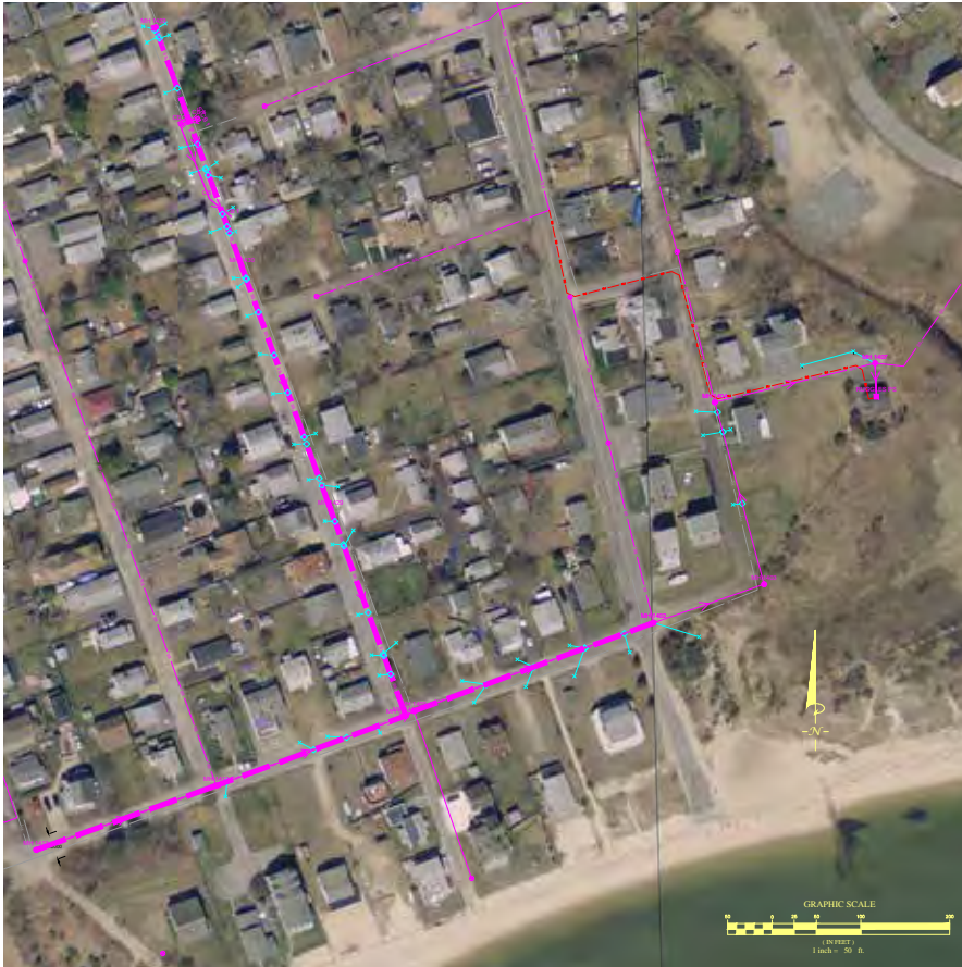
8-inch AC Pipe at Swifts Beach is permanently under water table at 17 feet depth
