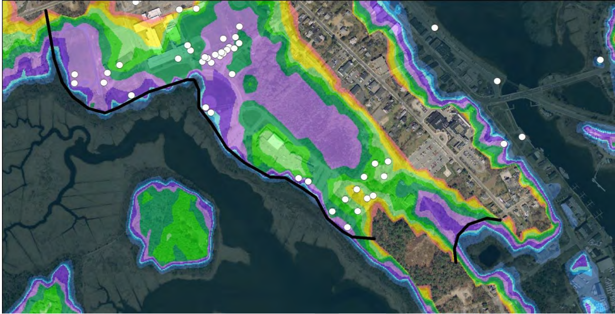
Figure 4-32. Potential earthen berm locations to reduce the flood risk for the Wareham Middle and High School area.
