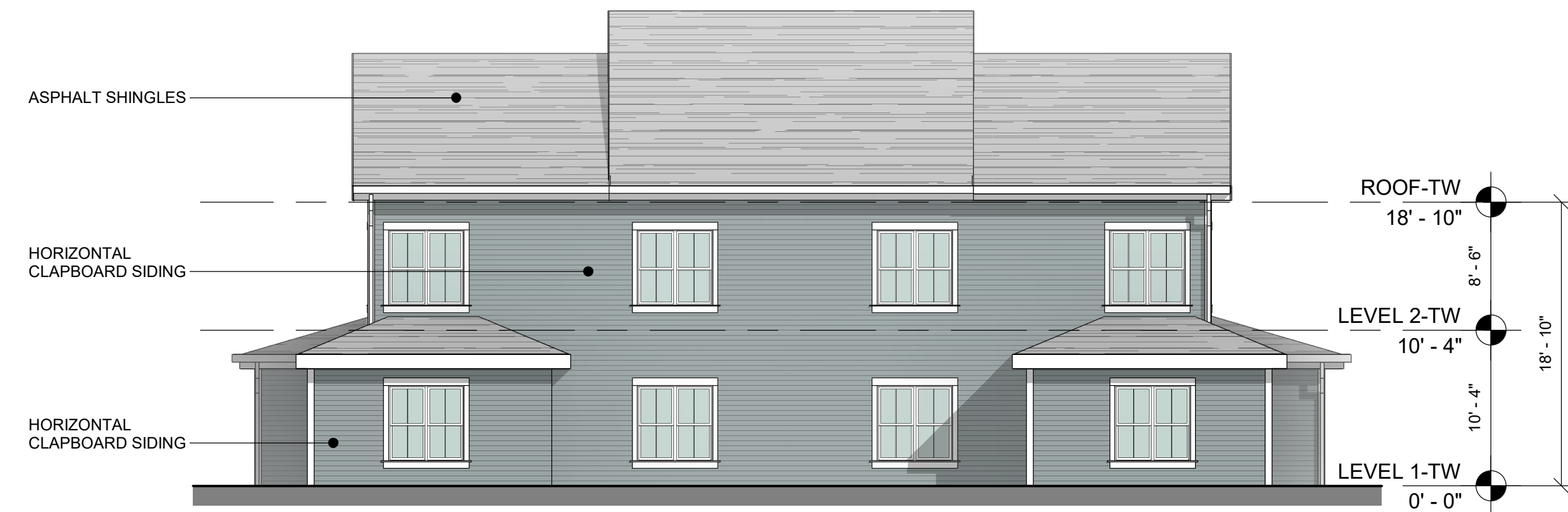
20 TYPICAL BUILDING-NORTH ELEVATION Scale: 1/8" = 1'-0"
