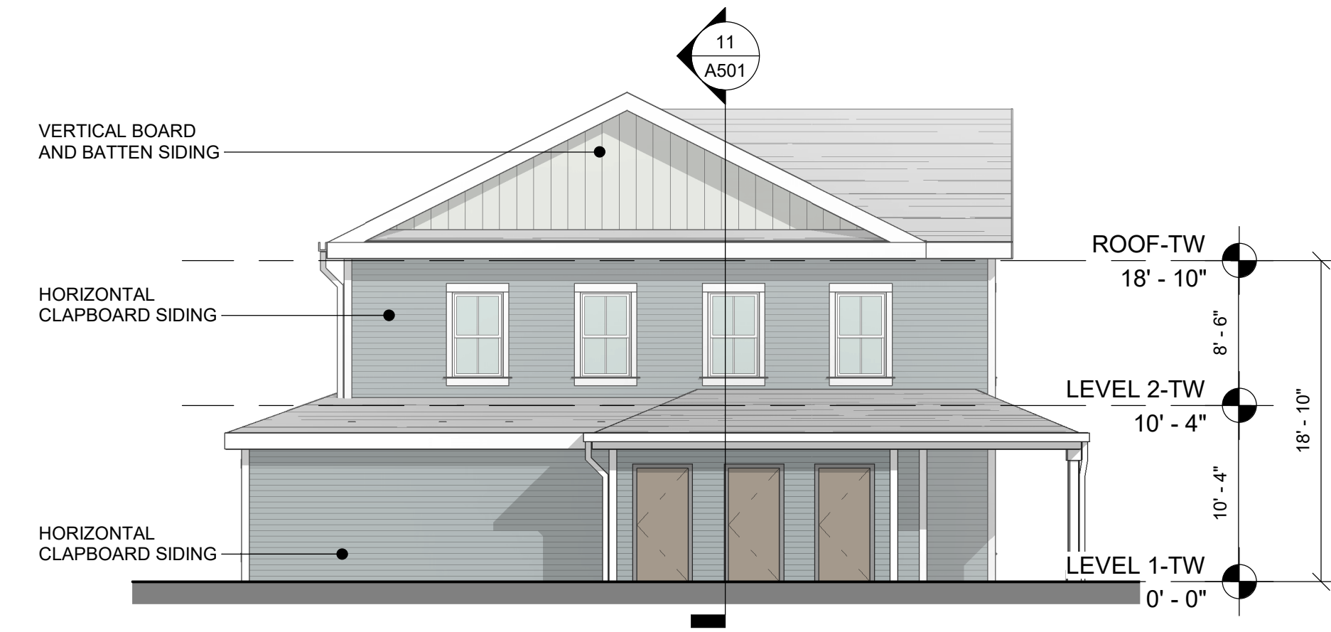
21 TYPICAL BUILDING-WEST ELEVATION Scale: 1/8" = 1'-0"
