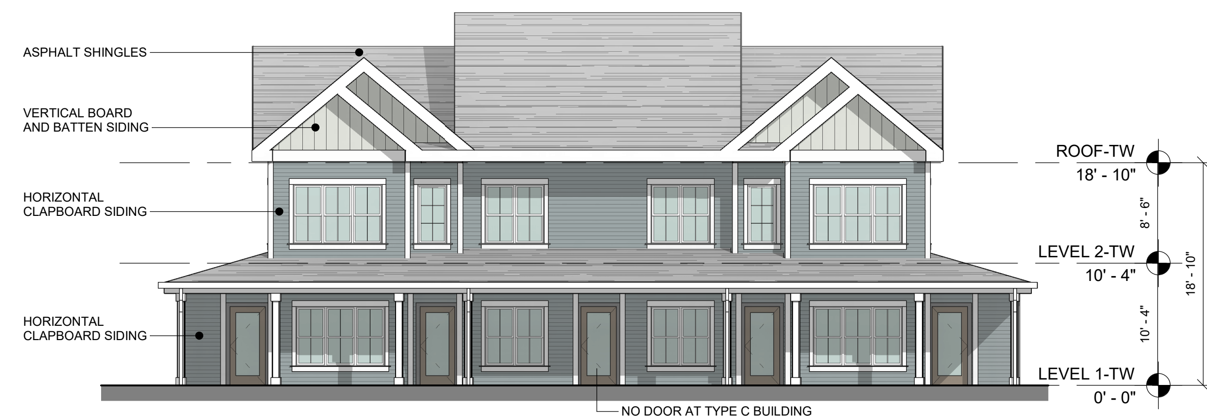
10 TYPICAL BUILDING-SOUTH ELEVATION Scale: 1/8" = 1'-0"
