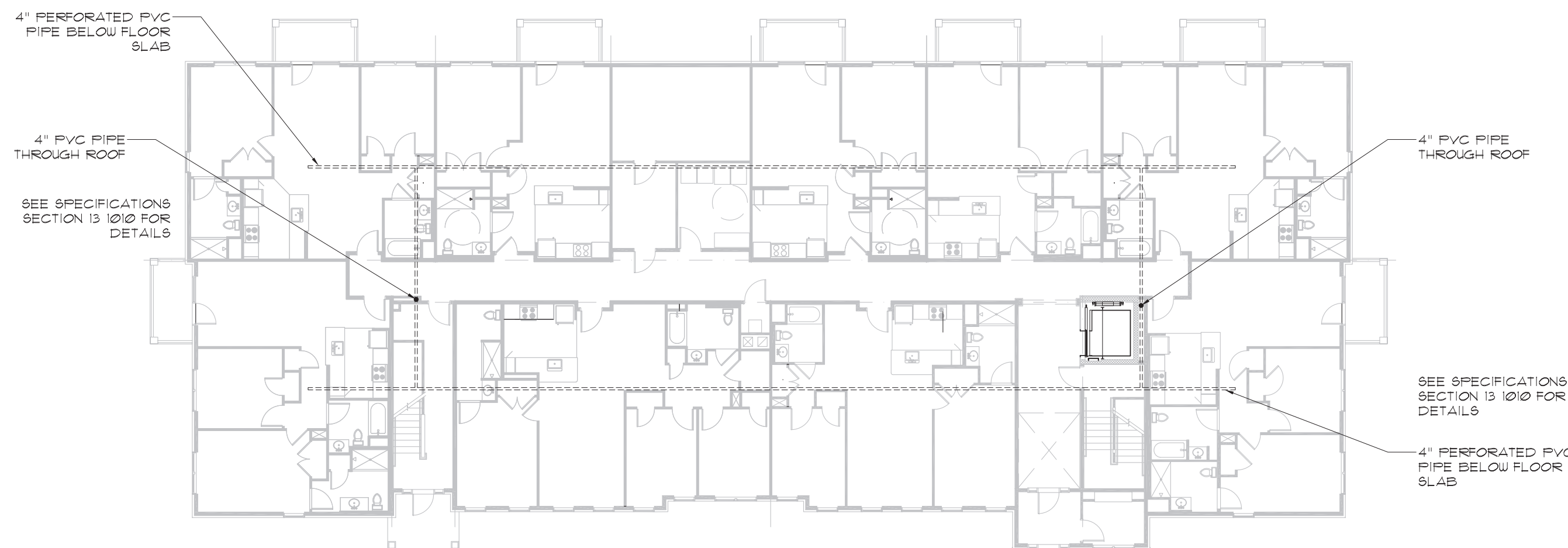
RADON SYSTEM PLAN, TYPICAL BUILDING F 3 N.T.S.
