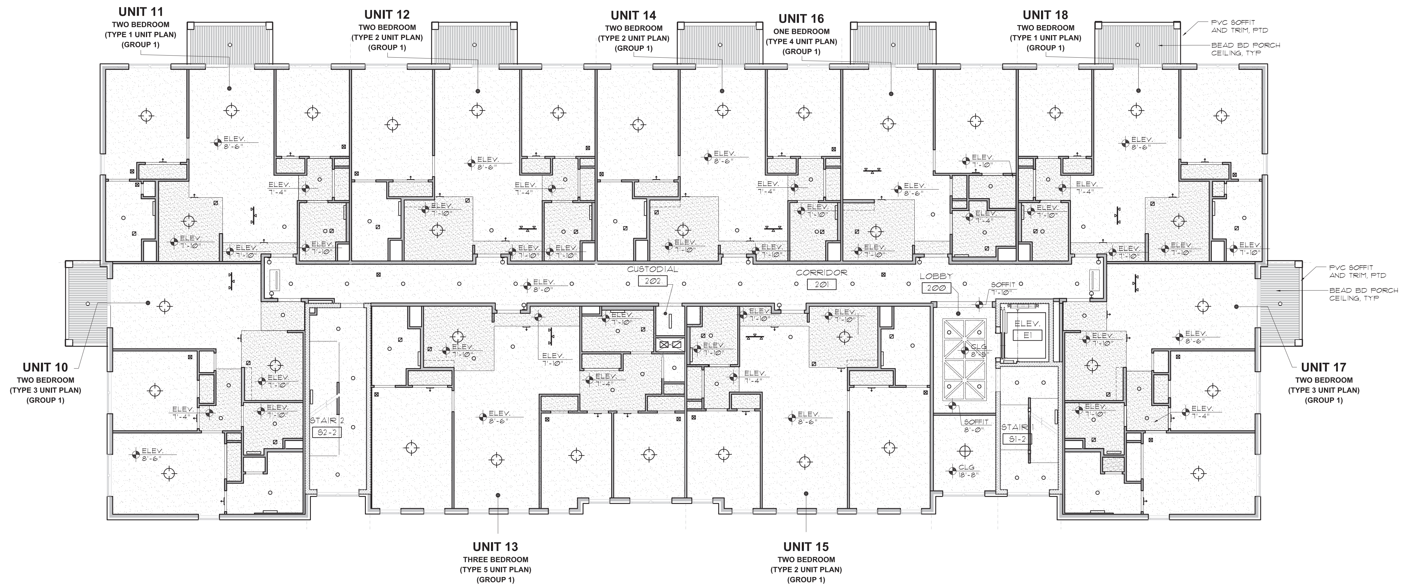
BUILDING E: SECOND FLOOR REFLECTED CEILING PLAN
