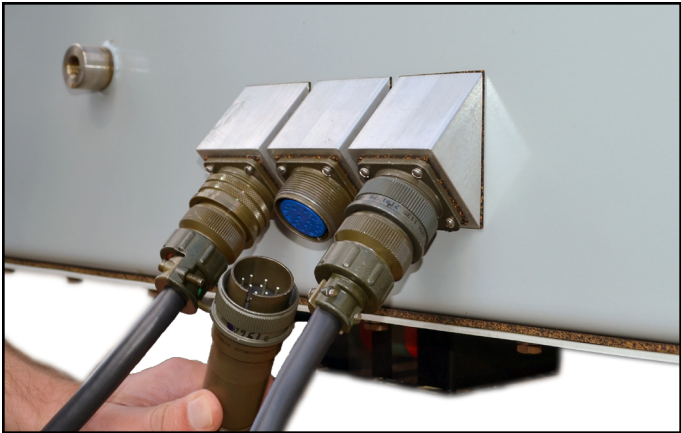
▲ Traditional configuration: 2-pin AC, 14-pin for control, and 8-pin 120VAC Voltage sensing connectors.
