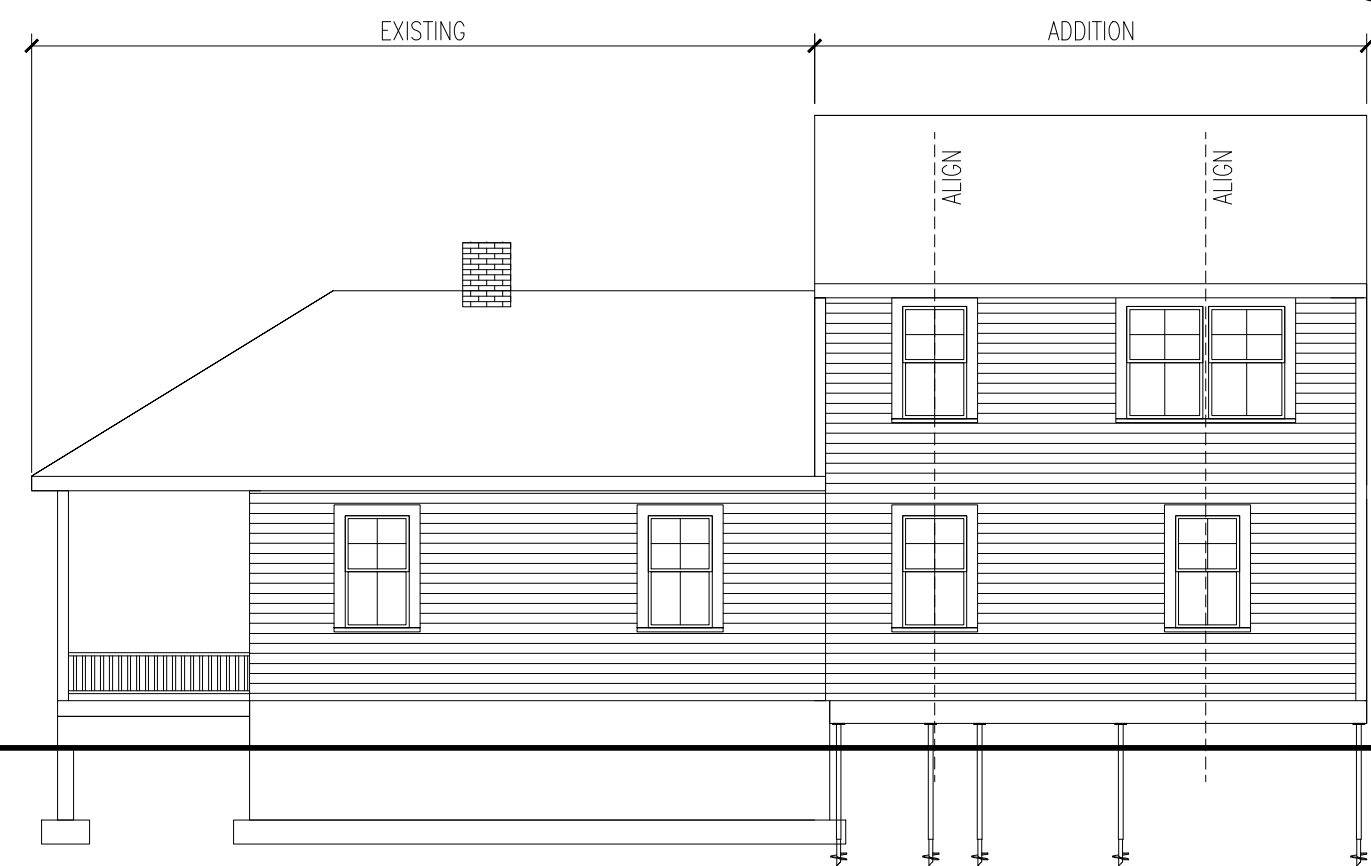
3 NORTH SIDE ELEVATION A-2.0 1/8"=1'-0"
