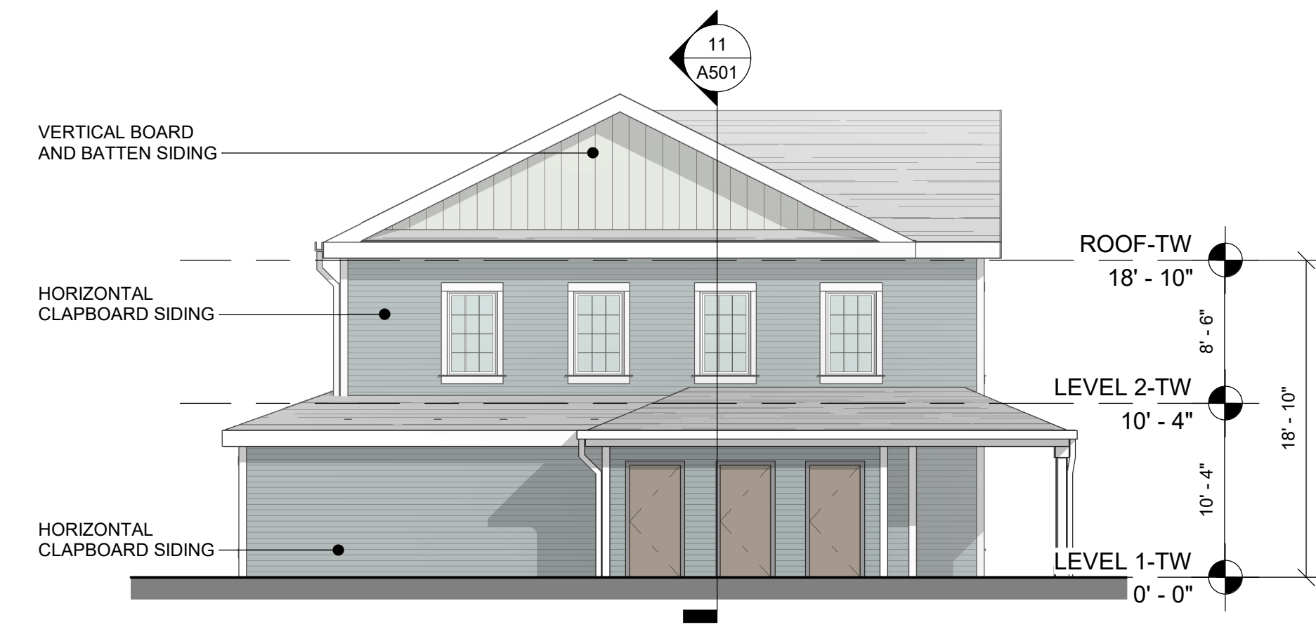
21 TYPICAL BUILDING-WEST ELEVATION Scale: 1/8" = 1'-0"
