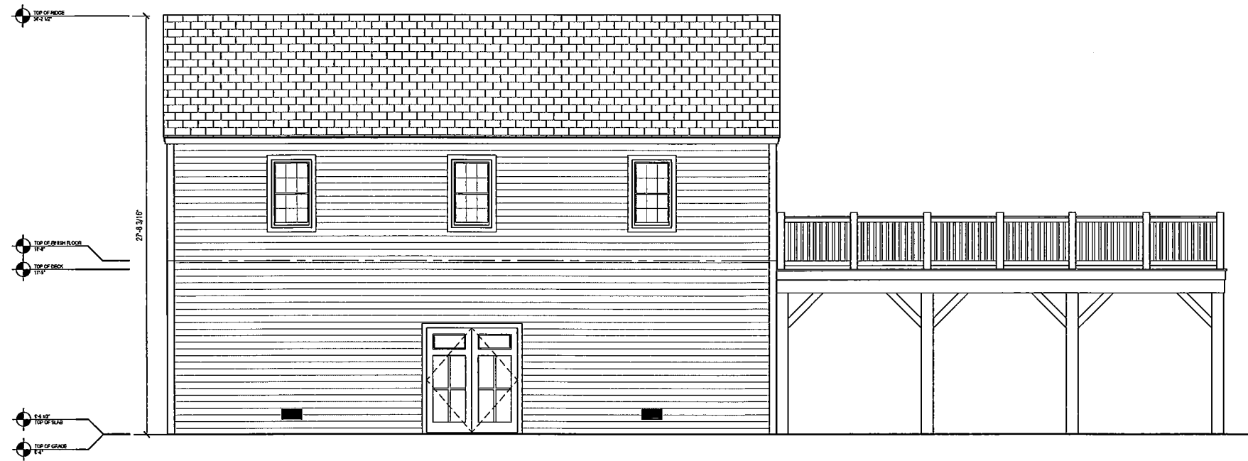
1 EXTERIOR ELEVATION - WEST 1/8" = 1'-0"
