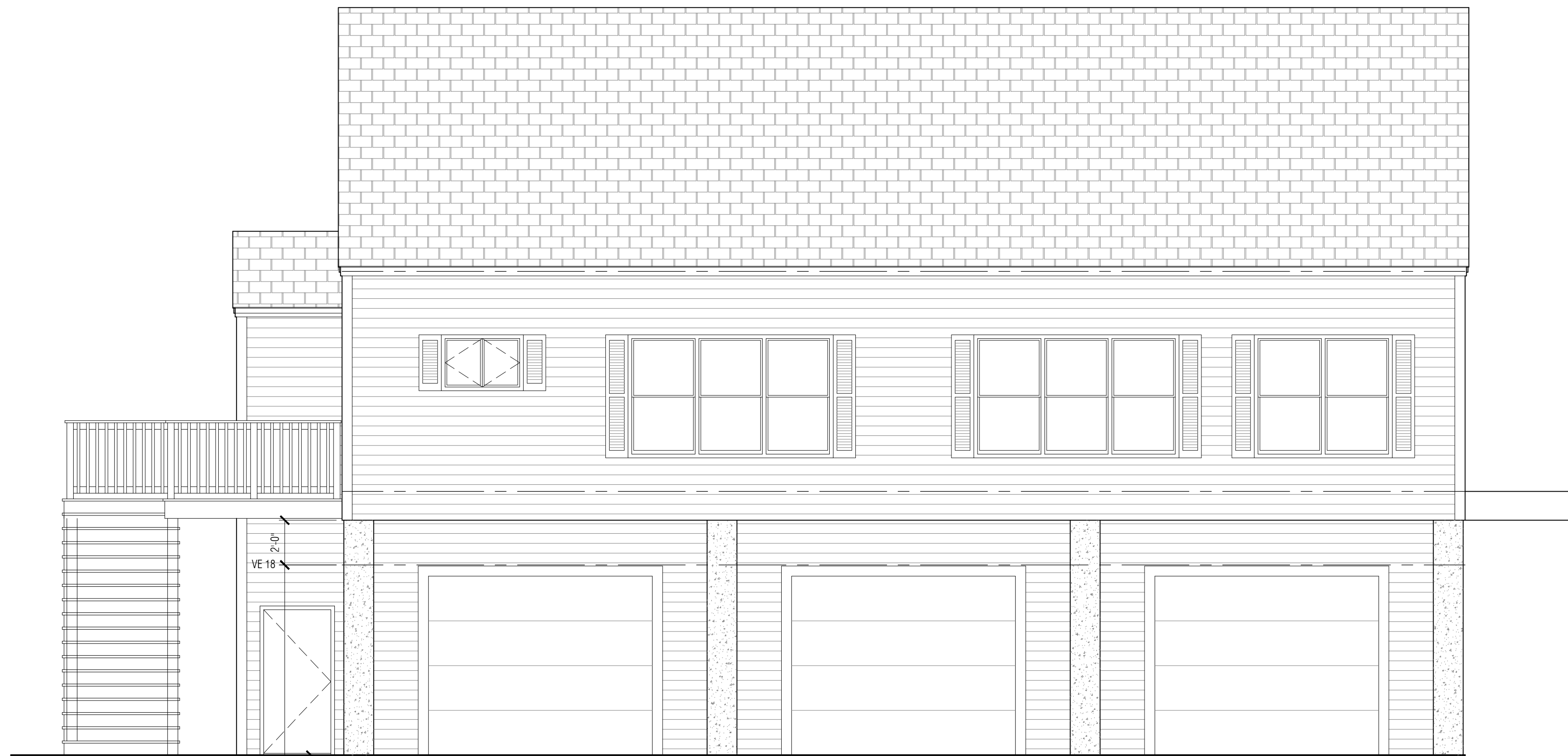
1 EXTERIOR ELEVATION - FRONT \frac{1}{2}'' = 1'-0''
