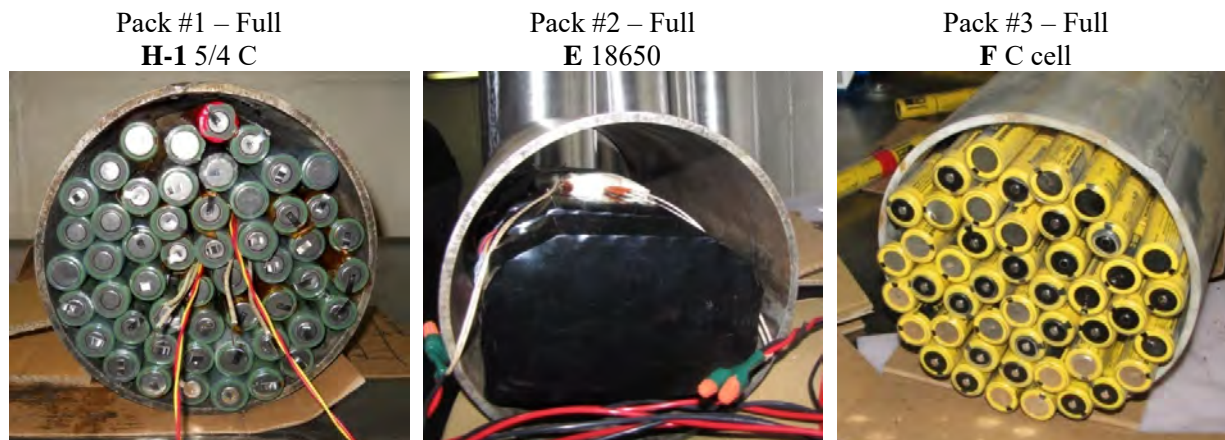
Fig. 13 — Typical battery stick and 63-cell module loading configurations
