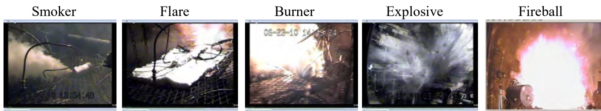
Fig. 4 — Single cell reaction classifications
