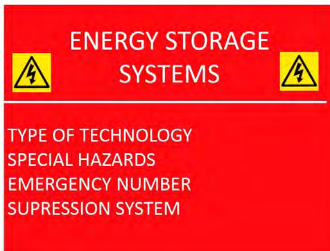
Figure B1 – Example of ESS Signage
