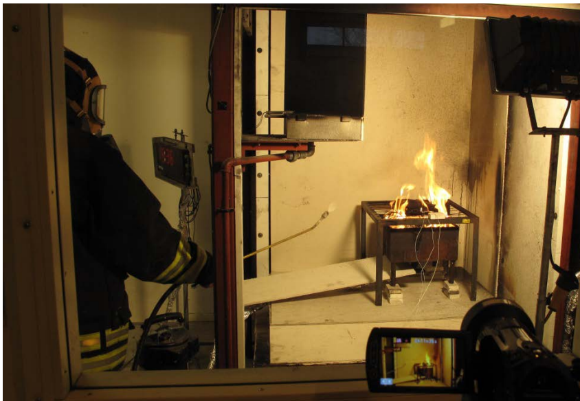
Figure 7 Applying water test 3
