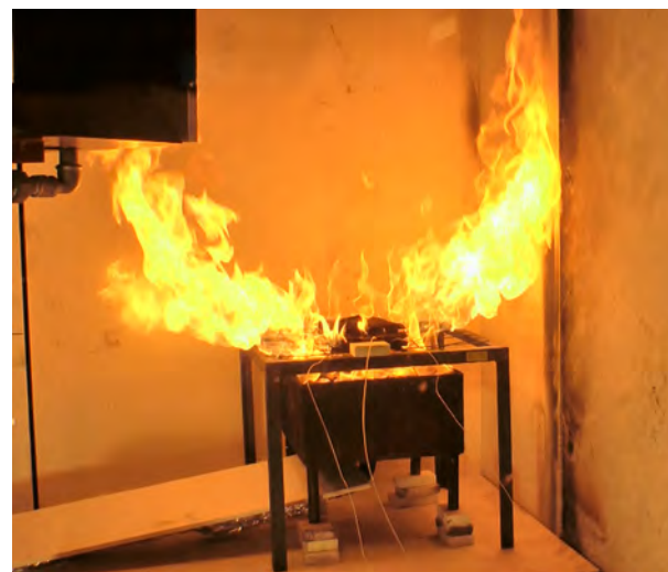
Fig. 6. Outbursts from EIG 100% SOC (test 1).
