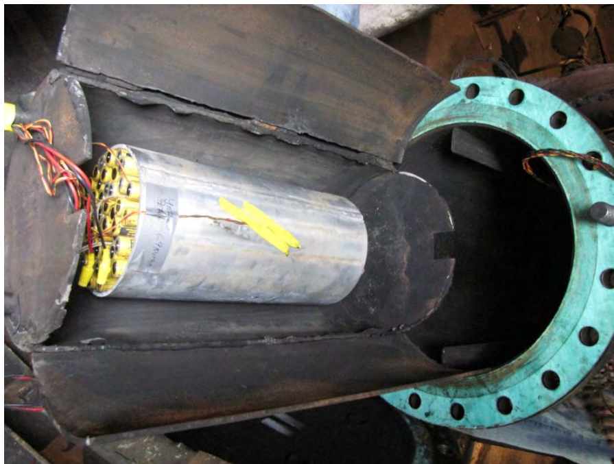
Fig. 14 — Pressurizable containment configuration
