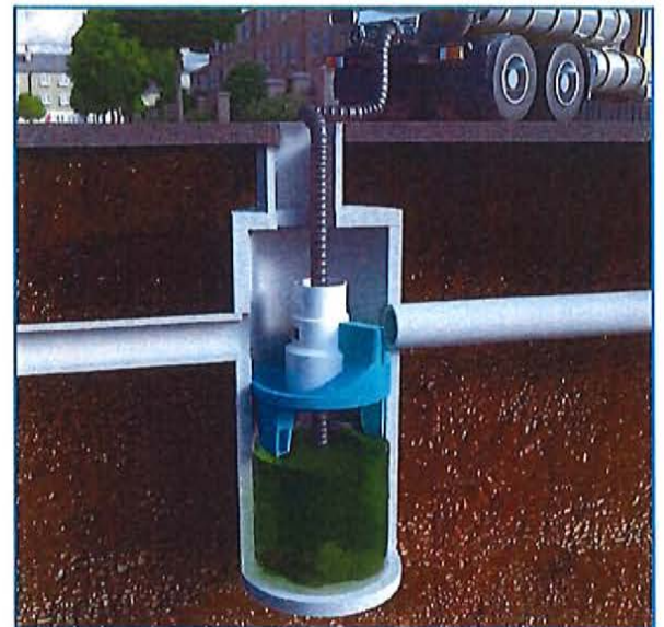
Fig 3. Maintenance is done with a vector truck
