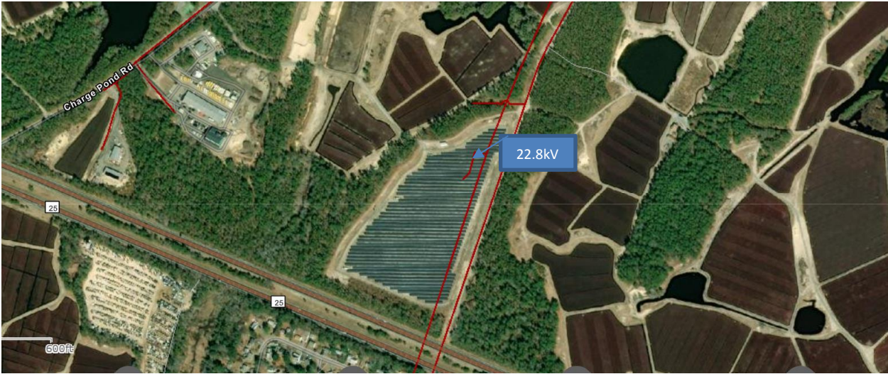
Figure 4. The BlueWave solar facility closest to the Project site: The red line indicates an above-ground line, the rating of which is 22.8kV.
