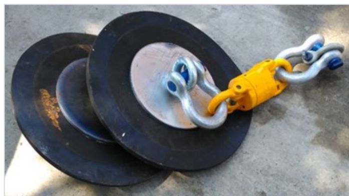
Illustration 14: Rubber discs with swivel
