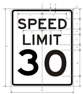
Fig. 9-1: Standard R2-1 (Speed Limit) Sign with Dimensions (Source: Standard Highway Signs, 2004)
