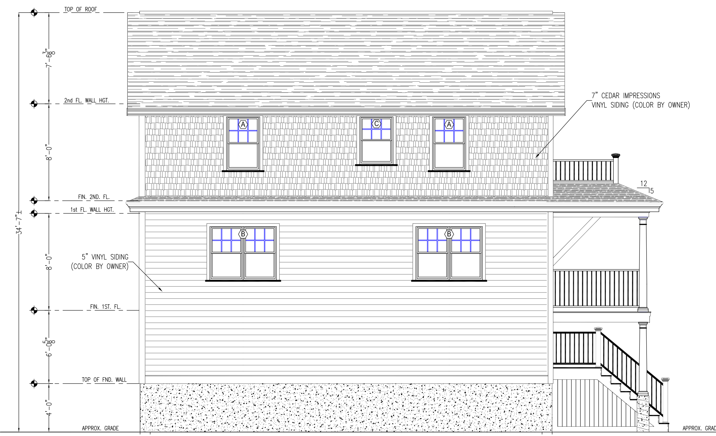
LEFT SIDE ELEVATION SCALE: 1/4" = 1'-0"
