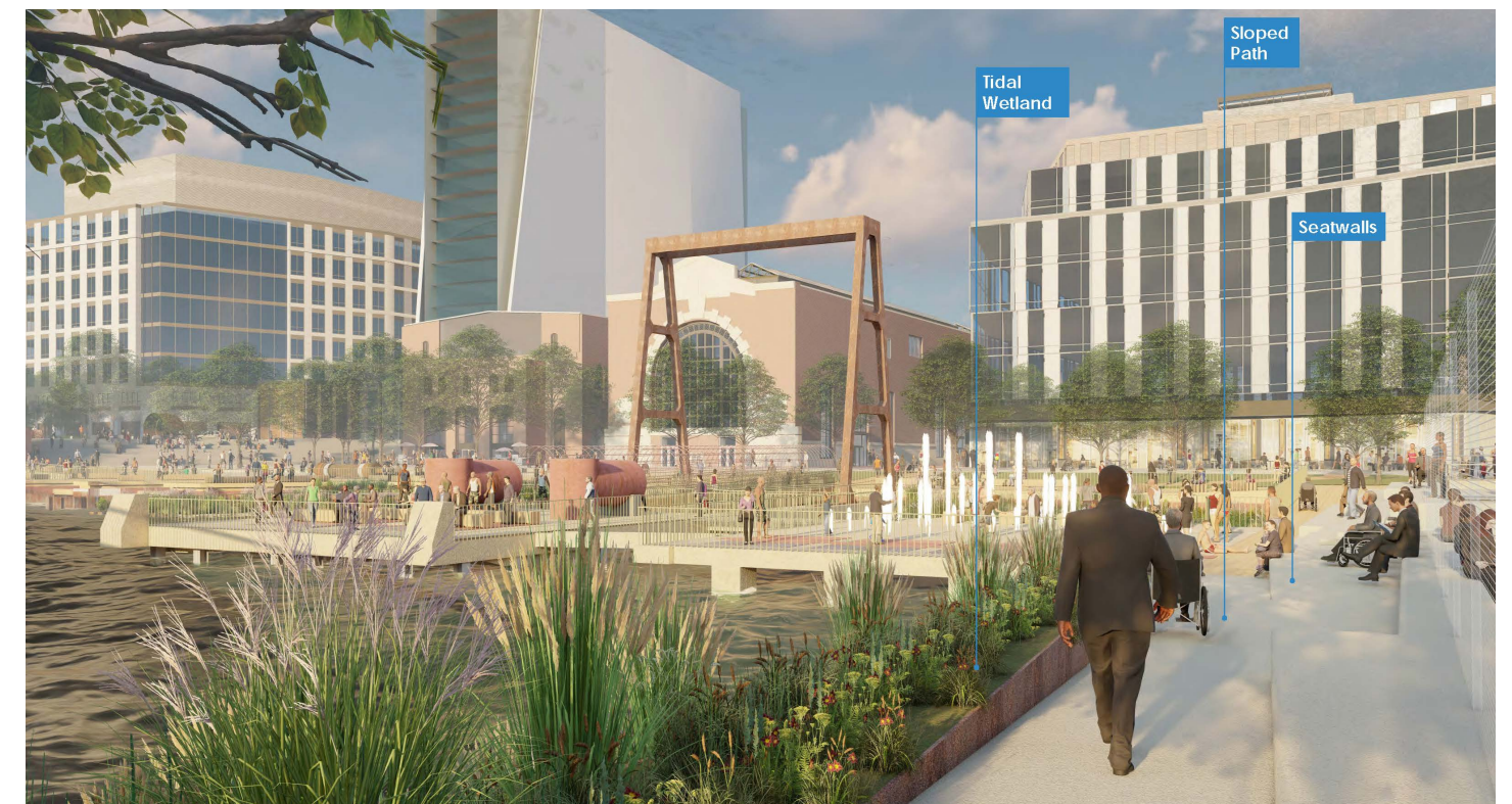
A tiered landscape is designed to accommodate the ebb and flow of storm surge and tidal flooding using natural wetlands to absorb and filter water.
