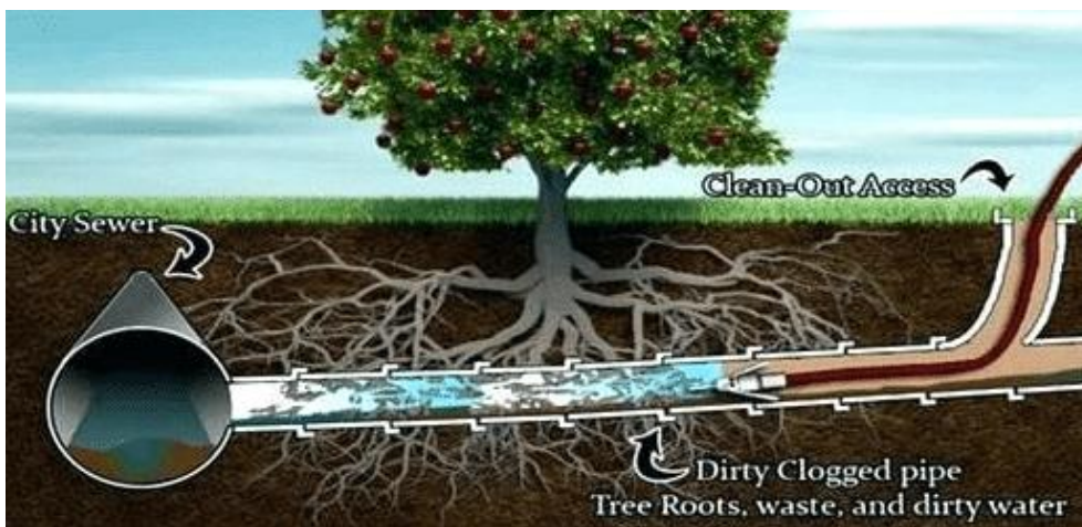
Figure 1: Small Diagram to Show Tree Roots in a Sewer System
