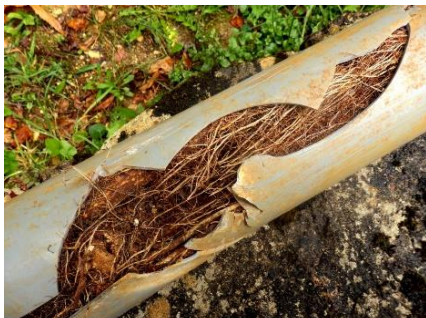
Figure 2: Real Tree Roots in a Sewer Line
