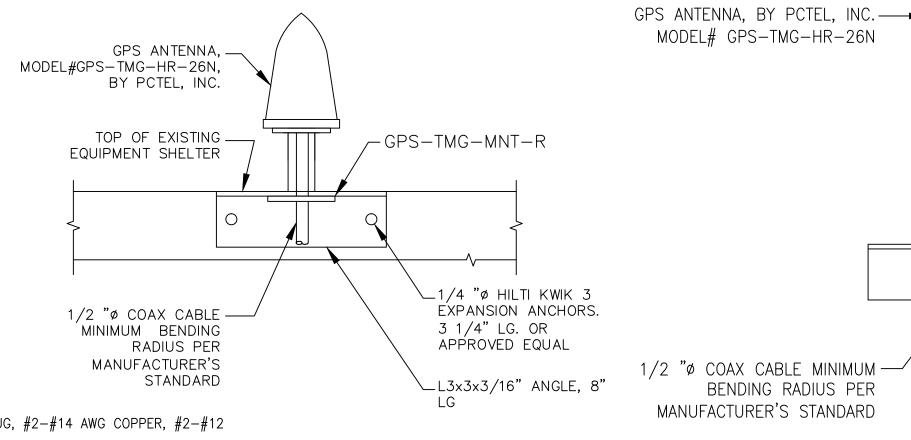
MODEL# GPS-TMG-HR-26N -L3x3x3/16" ANGLE, 8" LG ~3/8"ø U−BOLT 1/2 "Ø COAX CABLE MINIMUM BENDING RADIUS PER POST, TYP. MANUFACTURER'S STANDARD
